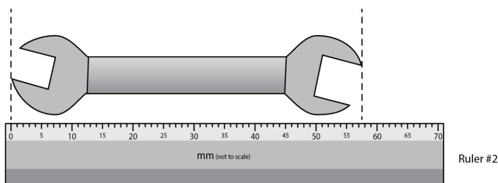
The smallest division on ruler #2 is 1 mm. If we now use ruler #2 to measure the spanner we can see that it lies exactly between the 57 mm and 58 mm divisions. So, we can confidently record a measurement of 57.5 mm.
