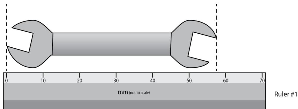
The smallest division on this ruler is 10 mm. The actual length of the spanner is 57.5 mm exactly. Using ruler #1 to measure the spanner it is hard to judge the length any better than to the nearest mm. We record a measurement of 58 mm.
