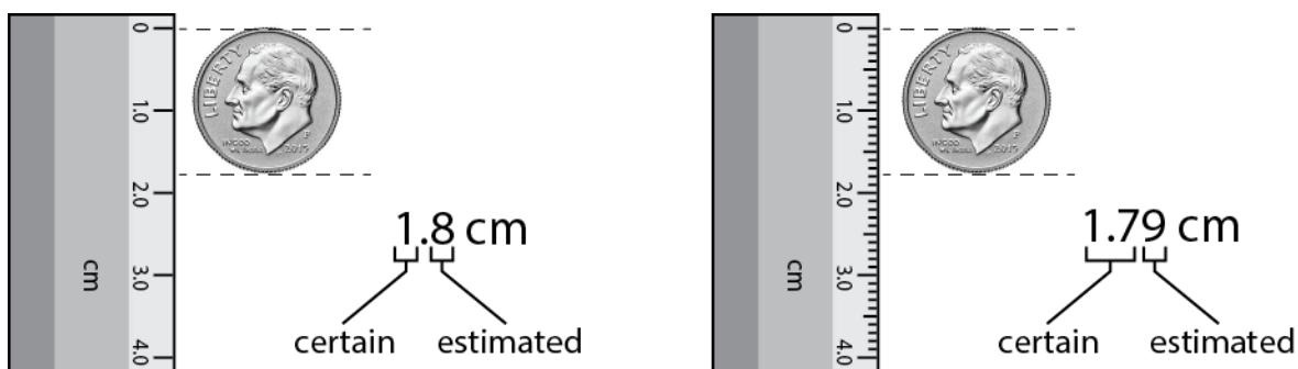
Here we are measuring a dime with 2 different rulers. The left-hand side ruler only has markings at every centimeter. The right-hand side ruler is more precise, it has markings every 0.1 cm.
