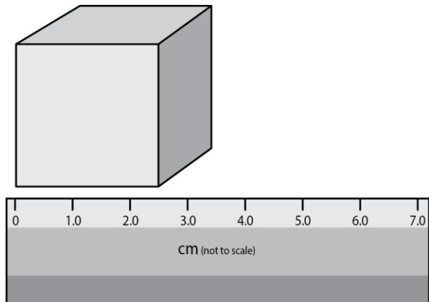
The edge of the cube is recorded as 2.5 cm long. This value has 2 s.f. When we do calculations with values we've measured, we always round the answer to the same number of significant figures as the measurement. First, let's do the calculation:
