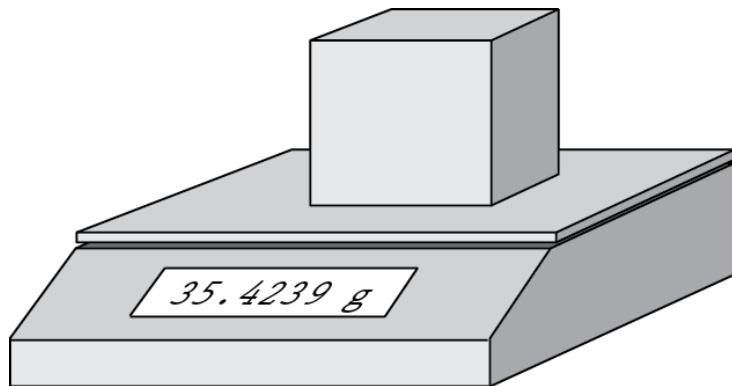
The balance gives us a value of  $35.4239 \text{ g}$  for the mass of the cube. This value has 6 significant figures.
