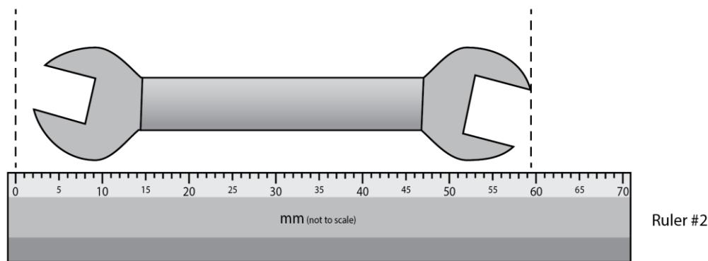
Many instruments will allow you to record a precise measurement, even if that measurement is not accurate. Let's imagine you measure the spanner with ruler #2, but don't carefully line up the end of the spanner with the zero mark. In this case, you record a precise measurement of 59.5 mm, however, this is several mm longer than the real length of the ruler. This measurement is *not* accurate, even though it is precise.
